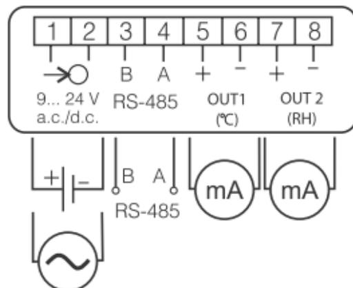
Transducer with current outputs
